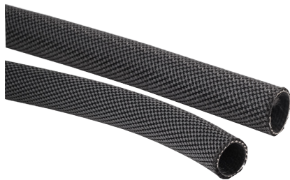
STABILO® hose, black Made of reinforced polyester yarn. Internal gumming of ozone and UV resistant EPDM rubber. The hose can handle temperatures from -30°C up to 80°C.
