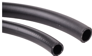
Base rubber hose The base rubber hose is made of PVC, nitrile rubber and polyester and has a smooth, black outer shell. Can handle temperatures from -20°C up to 60°C.
